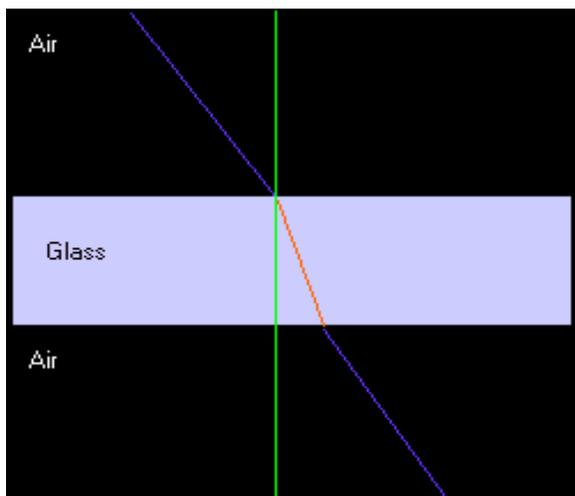
As can be seen from the above diagram the light ray actually is parallel to the incoming light ray, but is just moved slightly towards the normal. On the other hand if the light ray strikes an object that is in water, then transmits to glass and out to air, then that object contributes to the bending of the light rays.
