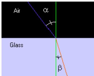
The purple line represents a light ray coming hitting a glass object and you can see that according to Snell's law that the light would bend towards the normal in this case (the red line).
