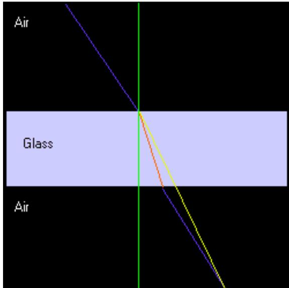
The lines above are all the same as in the previous diagram, except for the yellow line. This line represents the refraction index that is actually used since we are just interested in the end point of the ray.
